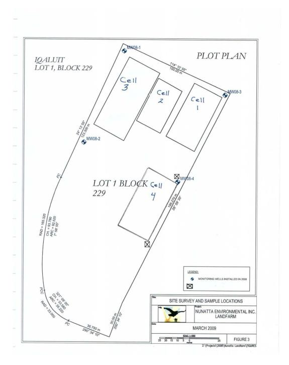
Black boxes with X at ends of cell 4 are locations for monitoring wells
