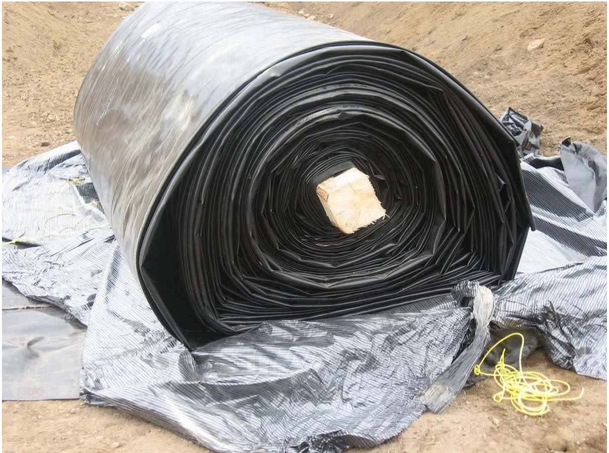
This is the new liner uncrated. Total weight 2200 pounds or 1000Kg
