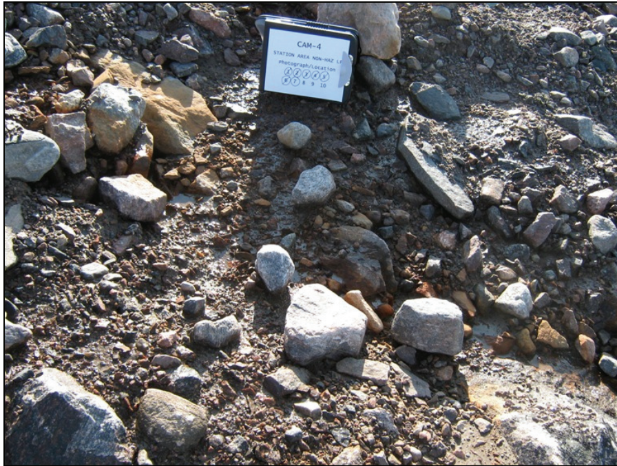
Photograph SNH-7B. Toe of slope near northeast corner. Orange staining and seepage discharging onto rocks at toe of landfill. Down-slope of photo SNH-12____ ↑
