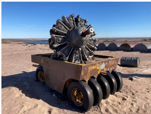
Figure 32 Ventura R-2800 engine in trailer at APEC 2, KW018 – Pelly Lake (Photo: Elsa Cencig, 2022).
