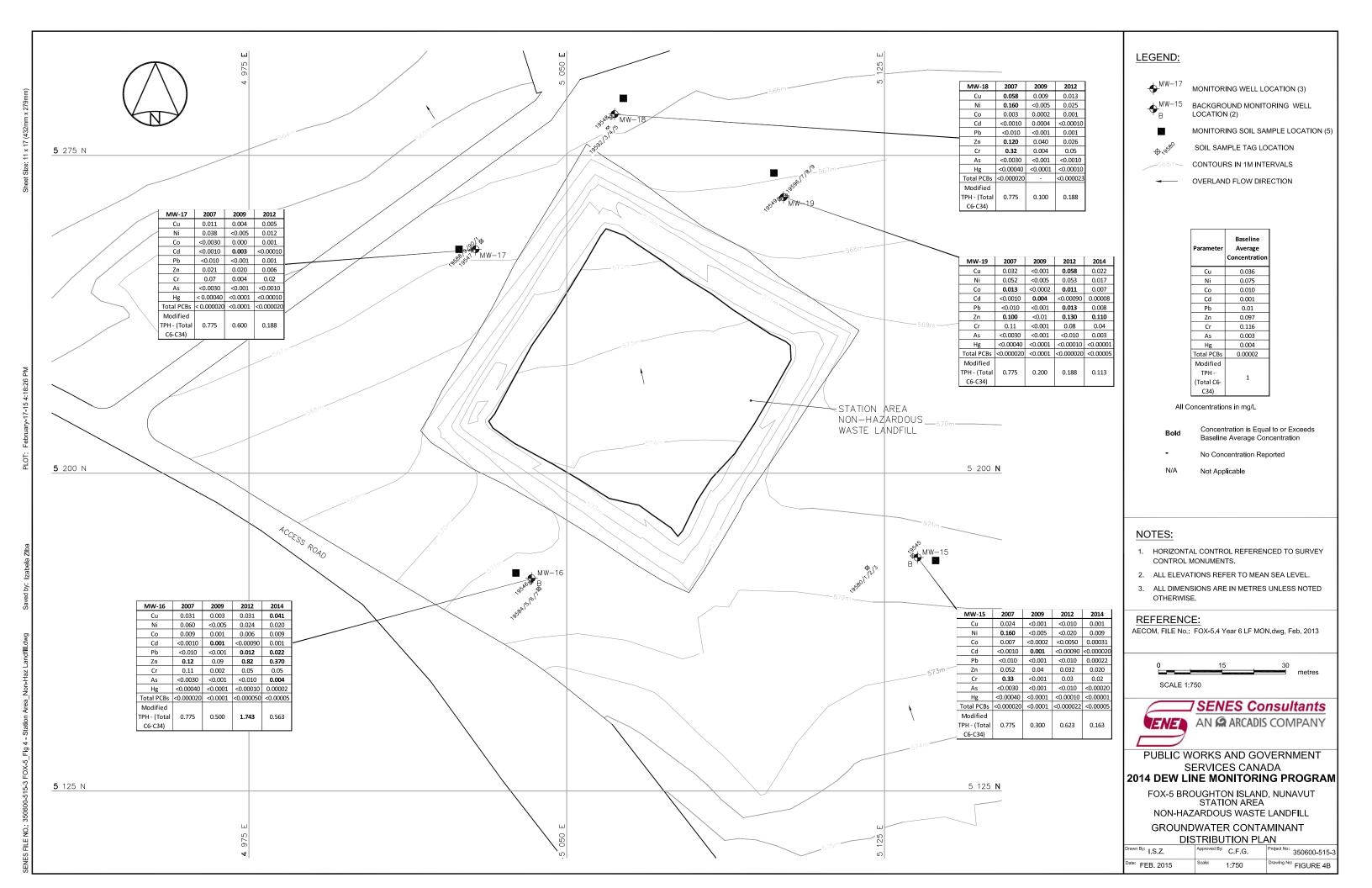
Groundwater monitoring was completed at five monitoring wells as shown on Figure 4. Groundwater monitoring and sampling at the Station Non-Hazardous Waste Landfill was generally completed as per the work plan. As indicated in Table 5.2, groundwater samples were not collected from two of five monitoring wells at this landfill as the wells had insufficient water. No duplicate groundwater samples were collected at this landfill.
