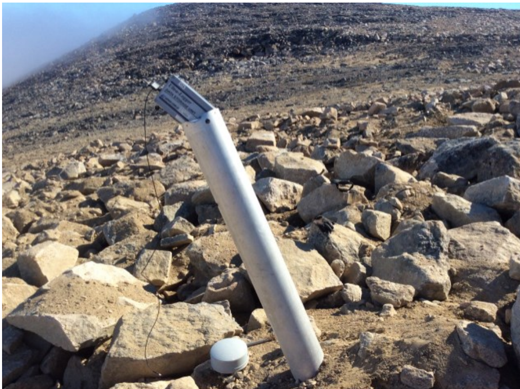
Photo 85: FOX-5 – Main Landfill – VT-4 – inclined 63 degrees to northeast (ATT119_Photo119.jpg)
