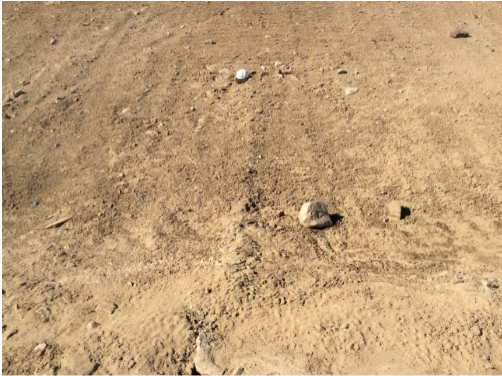
Photo 125: FOX-5 – Station Area NHWL – Southeast slope facing northwest – Feature H – minor self-armouring erosion with fines washed down slope (Acceptable) (ATT94_Photo94.jpg)
