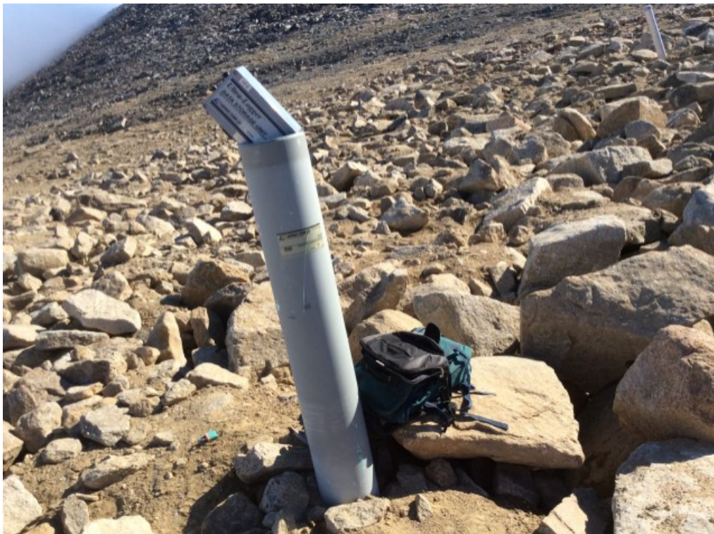
Photo 83: FOX-5 – Main Landfill – VT-2 inclined 77 degrees to northeast (ATT118_Photo118.jpg)
