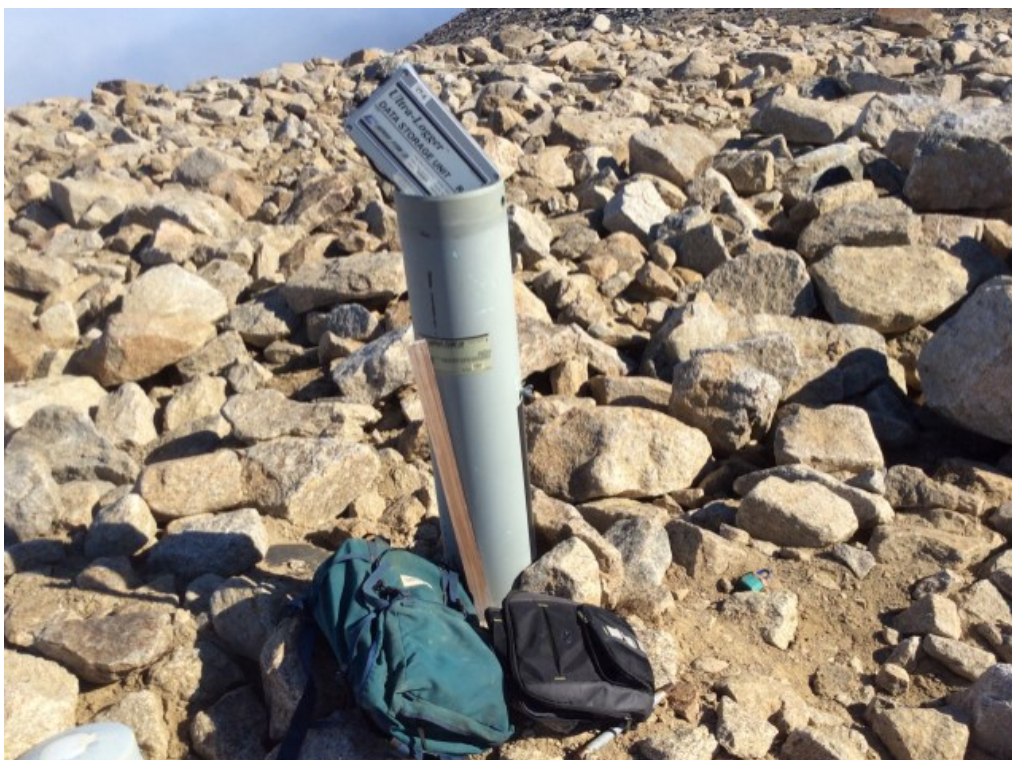
Photo 86: FOX-5 – Main Landfill – VT-5 – inclined 84 degrees (ATT120_Photo120.jpg)
