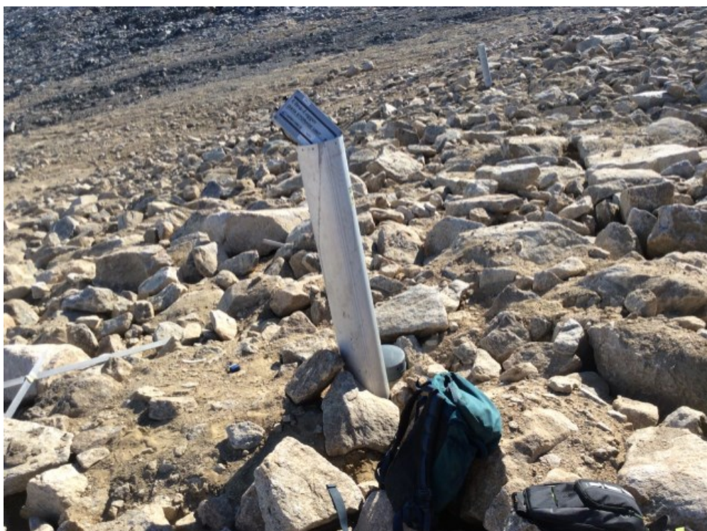
Photo 82: FOX-5 – Main Landfill – VT-1 – inclined 76 degrees to northeast (ATT117_Photo117.jpg)
