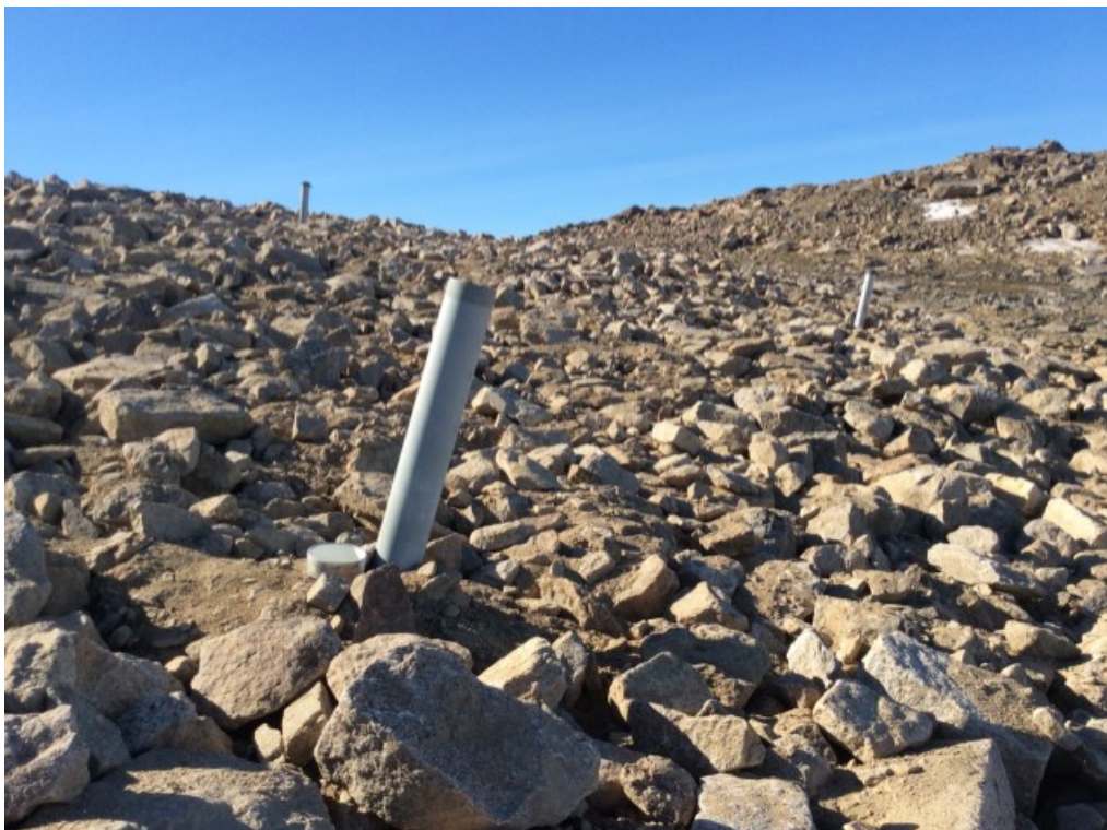
Photo 72: FOX-5 – Main Landfill – Feature A – Inclined thermistors facing VT-3 (ATT107_Photo107.jpg)
