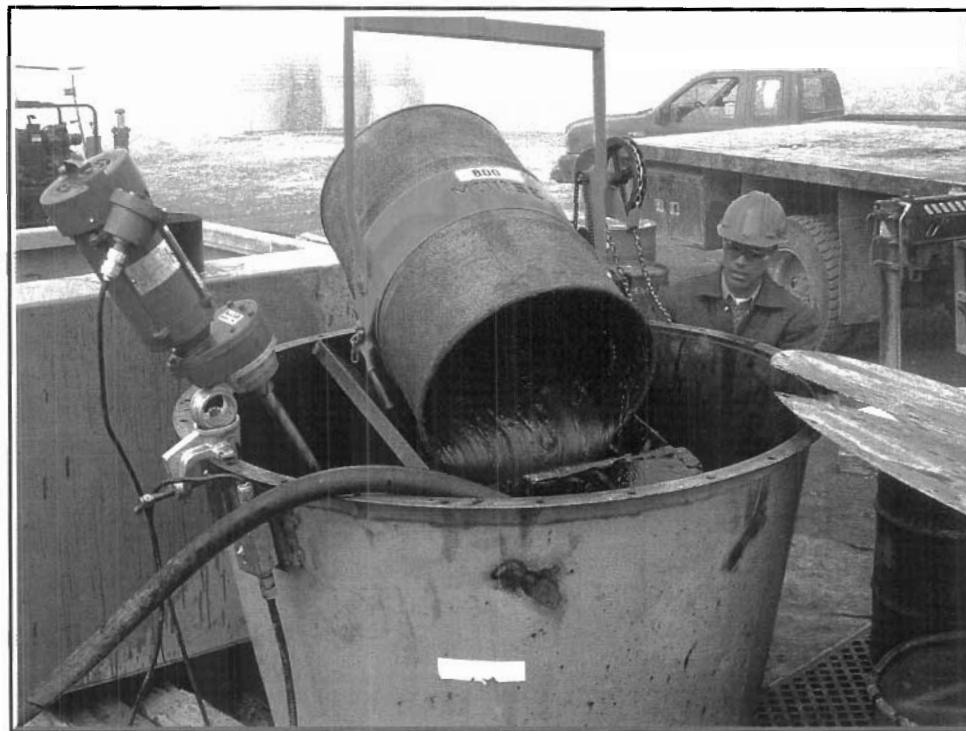
Photograph 6.1: Grease Drum Being Transferred to Mixing Tank
