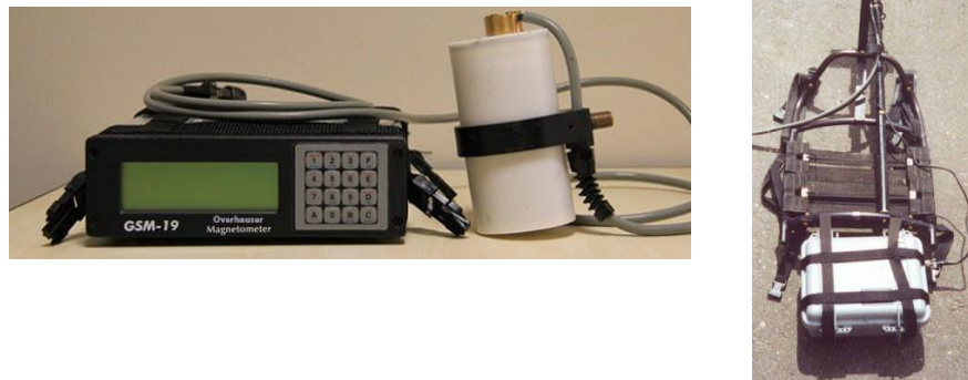
Figure 2: Overhauser Magnetometer setup.
