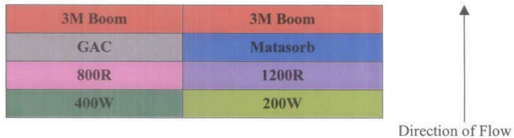
Figure VI-11: Arrangement of Filters and Sorbents in Filter Box September 2003 to June 2004 and Mass of PCBs Collected
