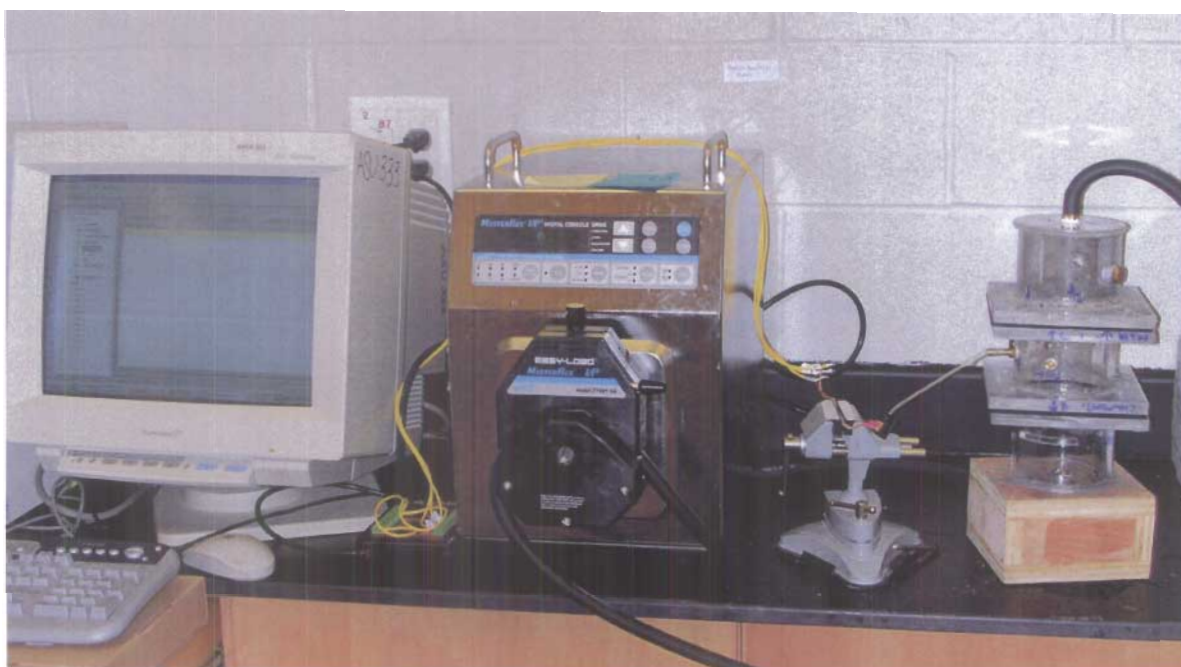
Photograph VI-18: The Experimental Set Up Including Computer, Pump, Pressure Sensor and Extraction Apparatus
