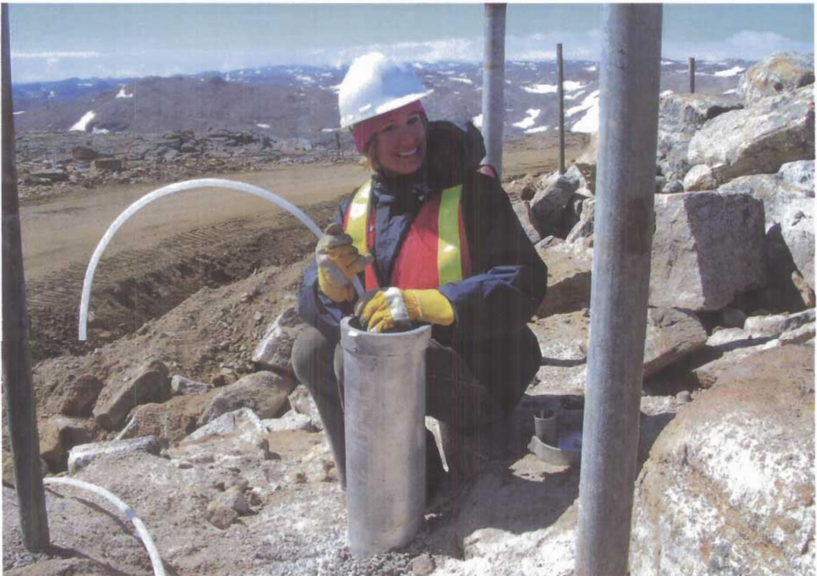
Photograph III-6: Paleah Preparing to Purge a Monitoring Well Prior to Collection of Water Samples
