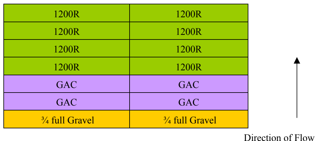
Figure 10: Arrangement of Filters in the Furniture Dump Filter Box at the End of the 2007 Field Season
