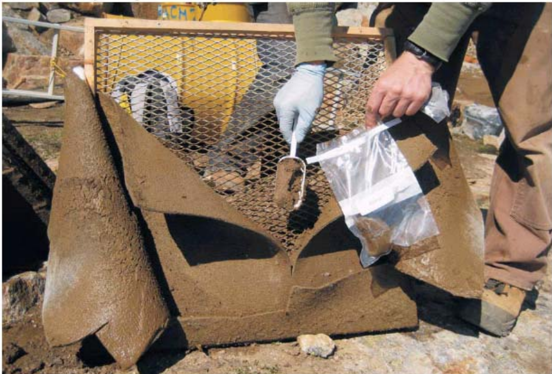
Photograph 19: Sampling Sediment From Between the Geotextile Filters After Having First Sampled the Filter
