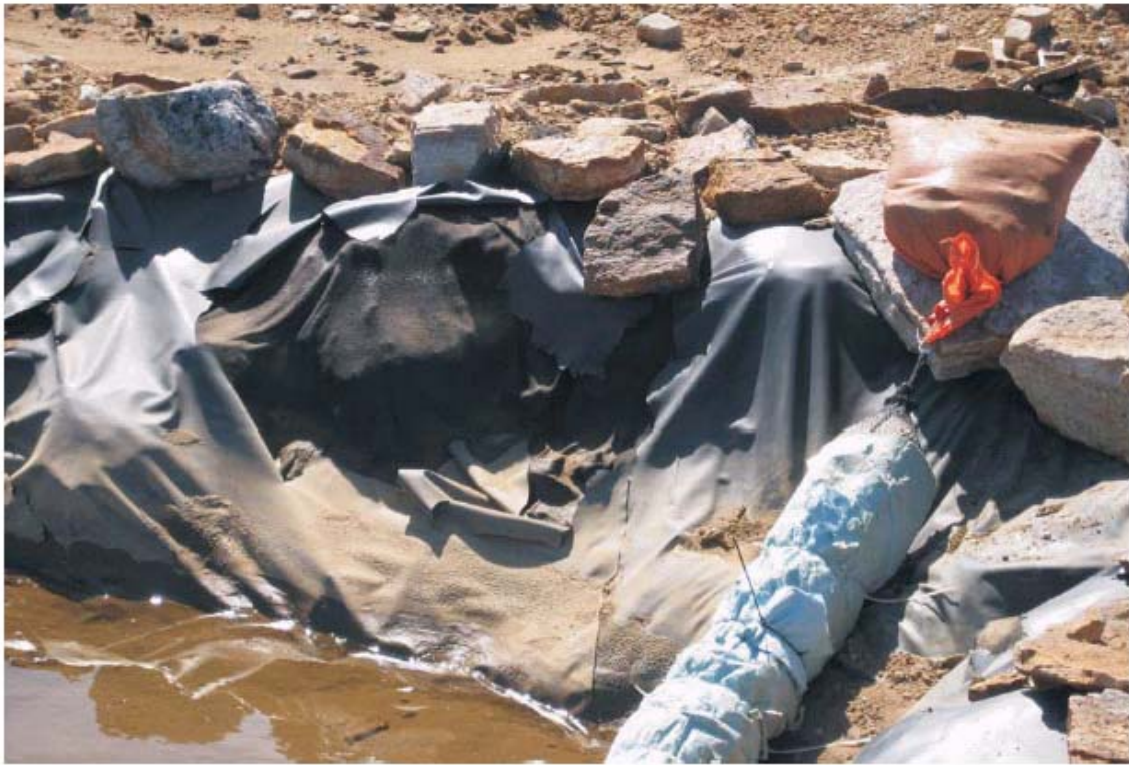
Photograph 12: The PVC Pond Liner Did Not Survive the Arctic Winter Above the Pond Level: Note the Damage Due to UV-Radiation and Weather
