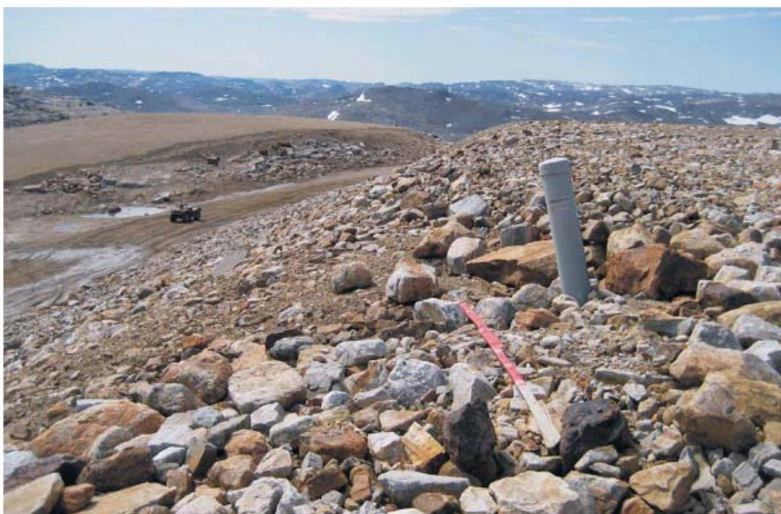
Photograph 4: The Tube Containing the Thermister String in the South Berm was Tilted; The Main Hydrocarbon Landfarm is Visible Across the Service Road
