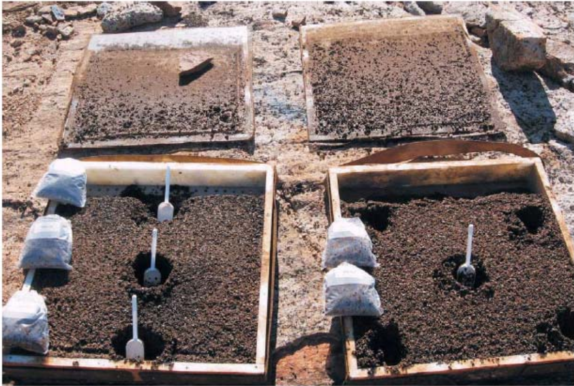
Photograph 18: Sampling a Cassette Containing GAC by Depth (Top, Middle and Bottom) and by Composite in Duplicate
