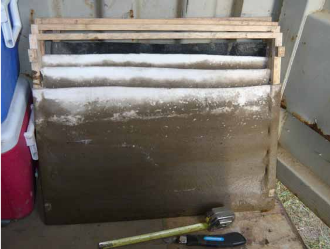
Photograph 22: A Set of Filters From the S1/S4 Beach Barrier Just Prior to Sampling
