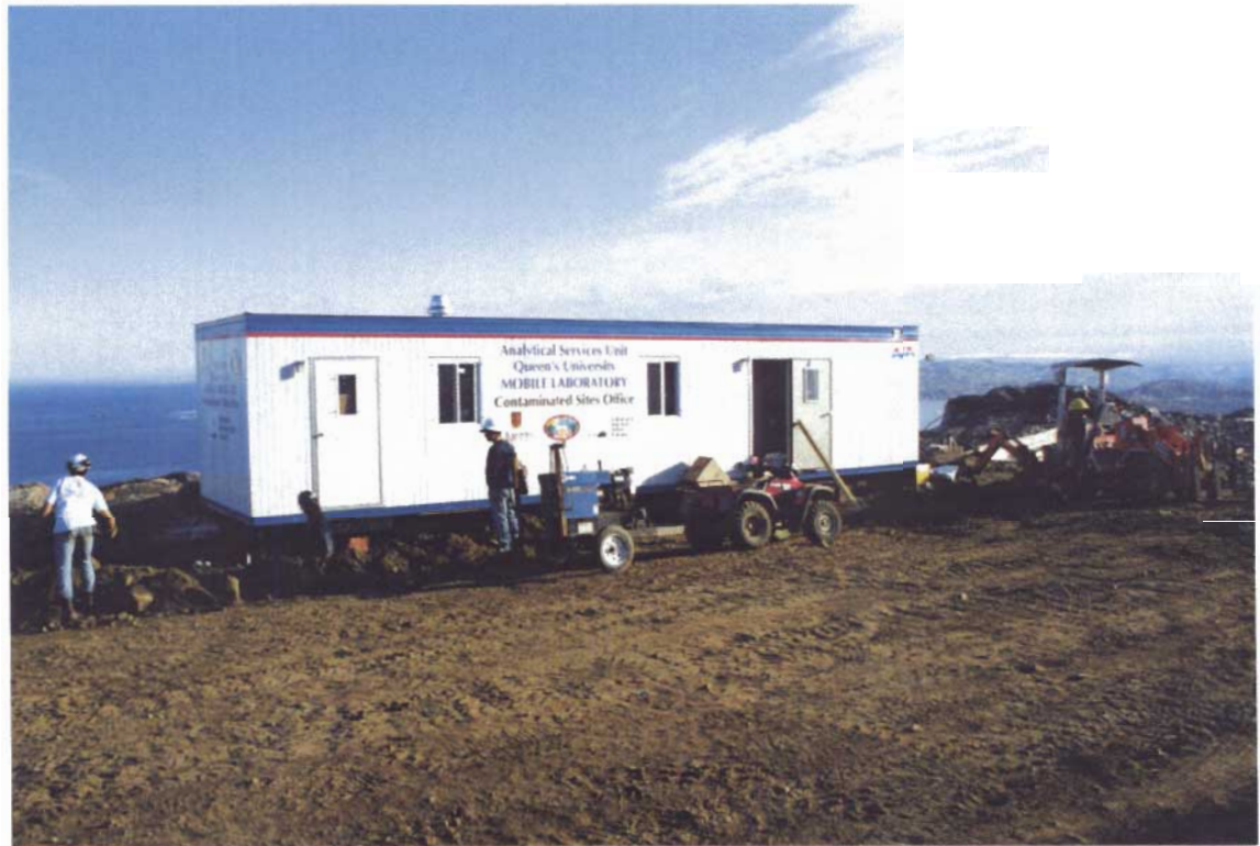
Photograph I-2: The Mobile Laboratory in Position at the Site; The Wheel Assembly was Removed and the Photograph Shows the Trailer Being Secured to the Ground.
