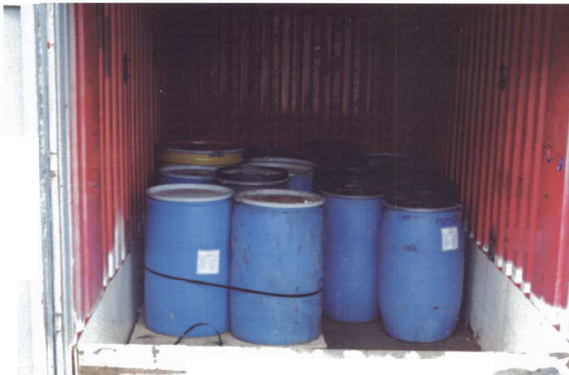
Photograph III-3: Blue Barrels Containing PCB-Contaminated Floor Tiles and Capacitors Inside Sea-Can #2.
