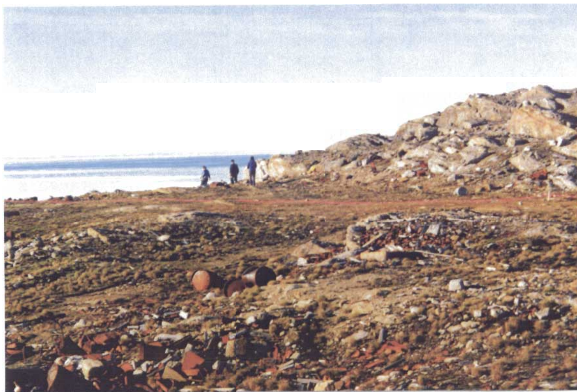
Photograph III-8: Sampling the Airstrip Dump: Ropes Were Set Out in a 10 Meter Square Grid on Top of the Dump
