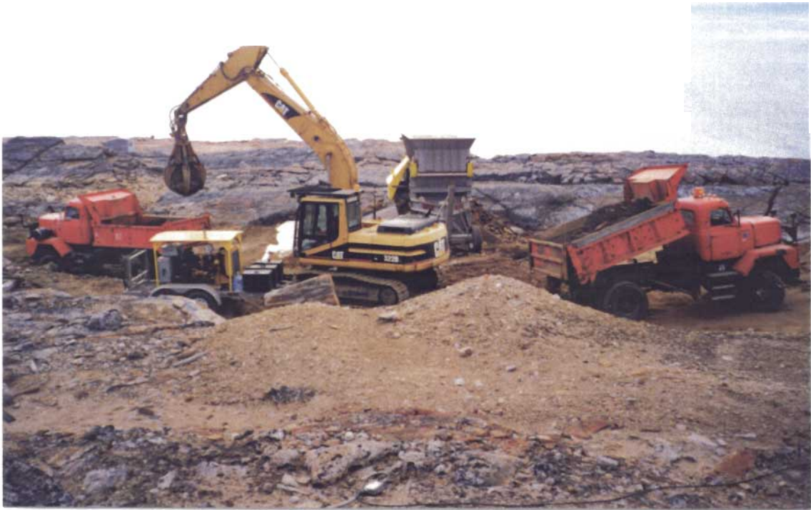
Photograph II-19: The Screening Plant on the Road Below S4 in Operation
