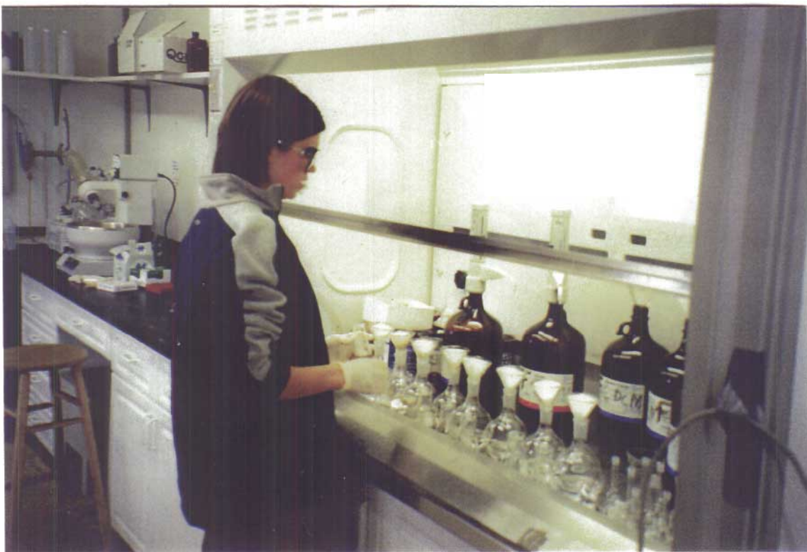
Photograph I-2: Conducting Analyses for PCBs in the Mobile Laboratory.
