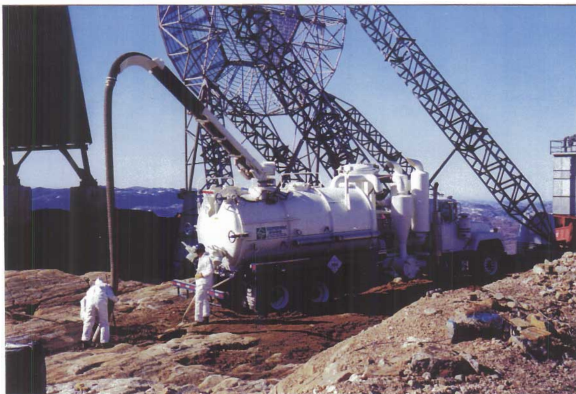
Photograph II-2: The New Vacuum Truck Removing Fine Material From Bedrock.
