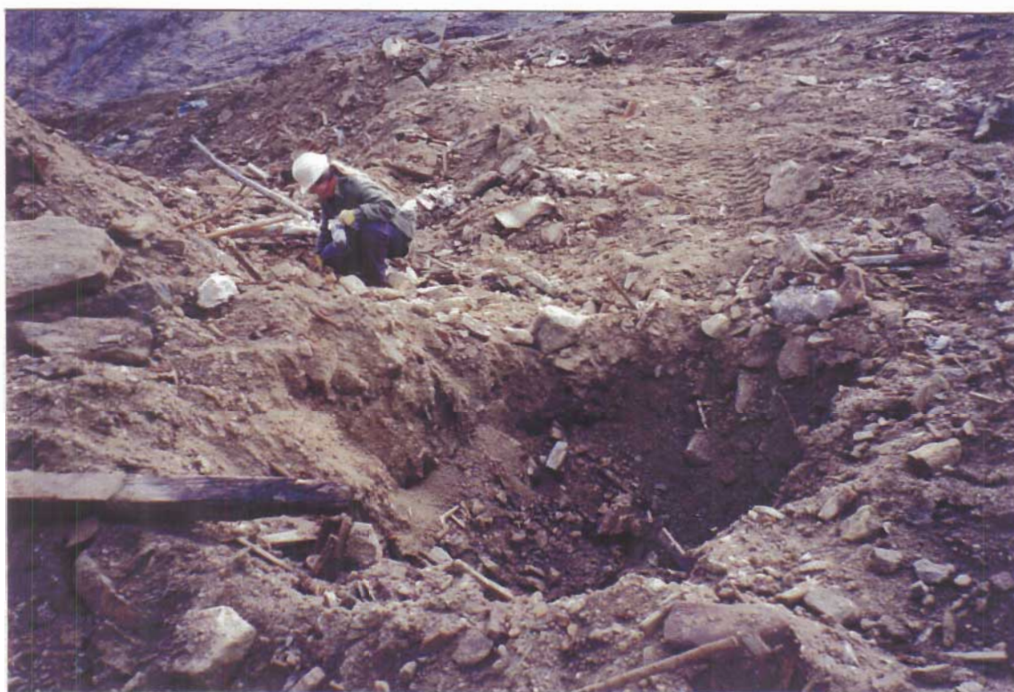
Photograph II-16: Taking Delineation Composite Soil Samples To Determine the Extent of Lead and PCB Contamination at the Beach Dump; The Hole was Excavated to Obtain Depth Samples.
