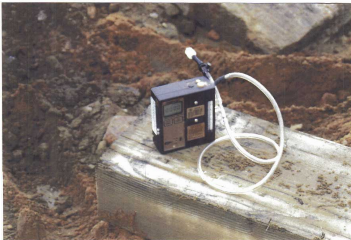
Photograph III-1: The Air Sampler Placed Near to Excavation Activities.
