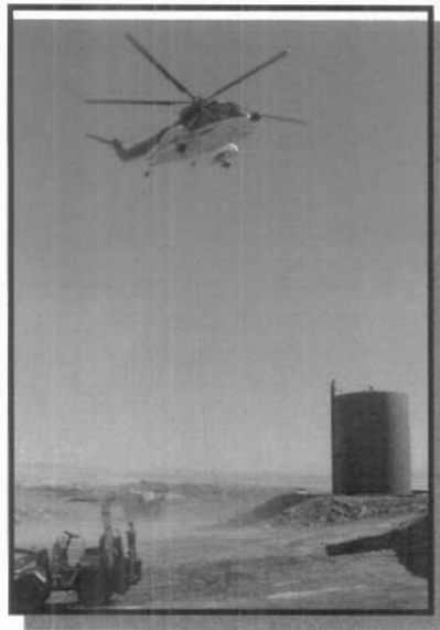
Photograph 2.2 Ground heater slung under Sikorsky S-61 helicopter
