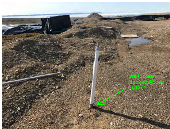
Photo 4 View of MW4 looking west (heaved well screen is visible)
