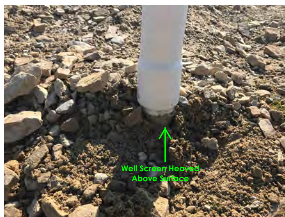
Photo 6 MW6 (heaved well screen is visible)
