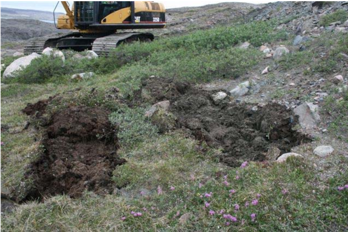
Test strips to locate tailings deposited at the location where the berm was breached. Strip on the left had no tailings. Strip on the right contained tailings
