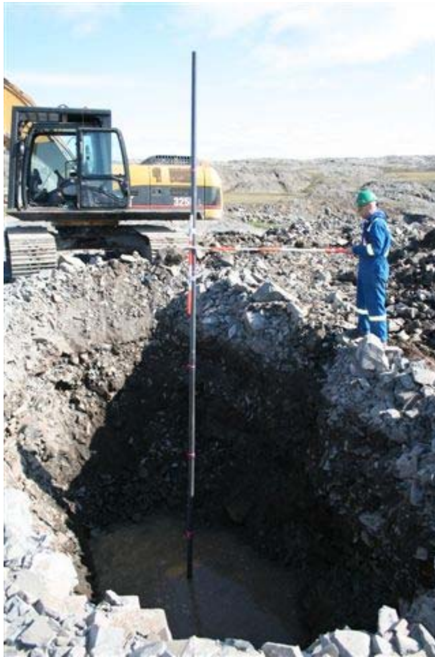
Thermistor at location "A". Marks on the pipe are at one meter intervals
