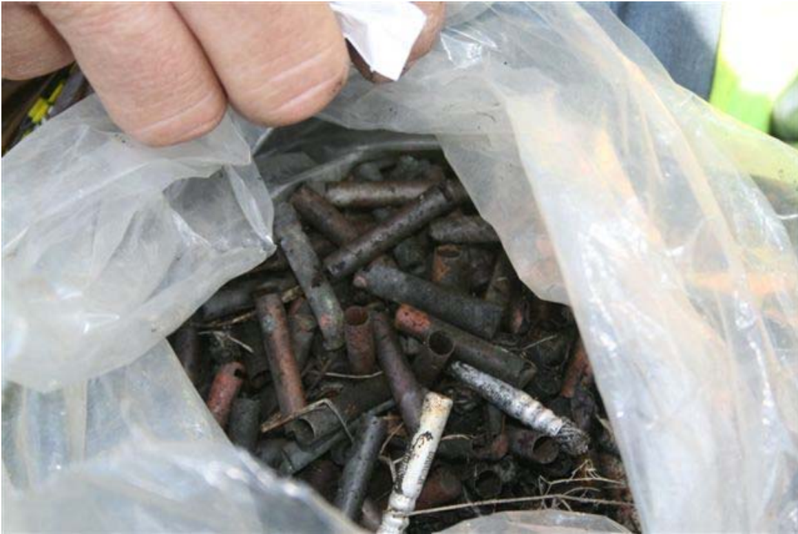
Blasting caps collected. Silver blasting caps are live.
