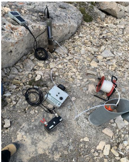
Photograph 1: Low-Flow Sampling at MW-3
