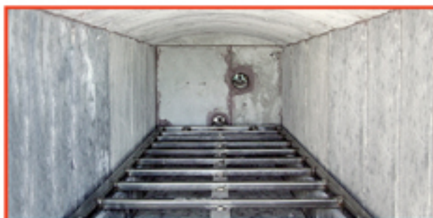
Inner walls made of high quality refractory cement resisting high temperature up to 1650°C.
