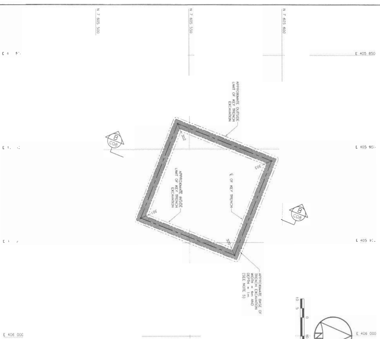
KEY TRENCH EXCAVATION PLAN
