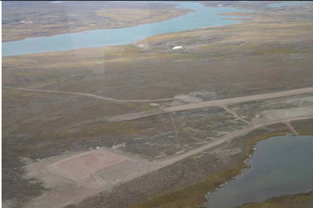
Photo 3. SSDF. Ponding areas can be seen on the southern side, near the corners, and on the northern side, near the access ramp. Direction photo taken: SW. Photo provided by INAC.
