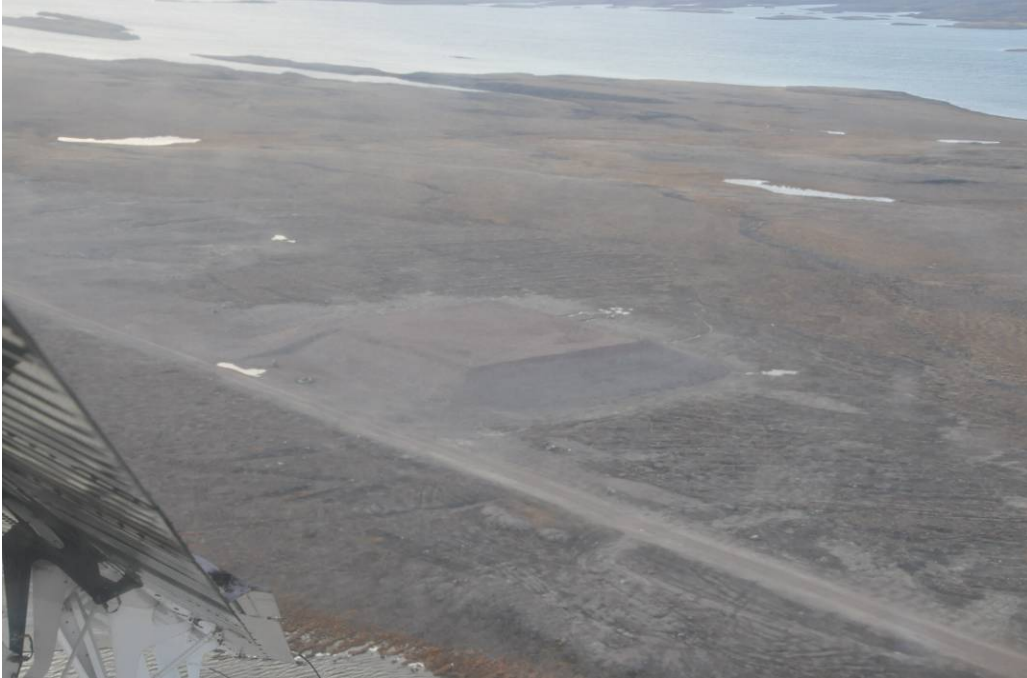
Photo 1. The CAM-F Secure Soil Disposal Facility (SSDF). Areas with ponded surface water can be seen at both the northern (left) and southern (right) toes of the SSDF. Direction photo taken: SSE (picture # DSC_0264).
