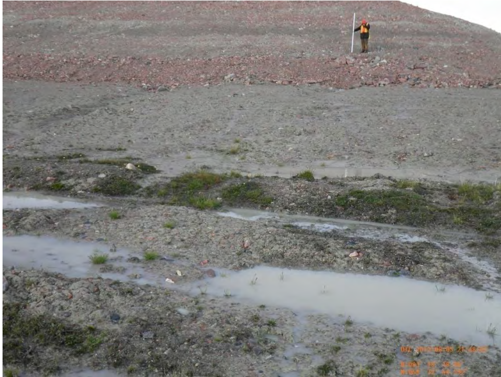
Ponded water from the active seep near the southeast corner of the SSDF. Viewpoint 84 (Figure A-2; Appendix A). Photograph reference RIMG0084 (CD-ROM). Direction photo taken: SE
