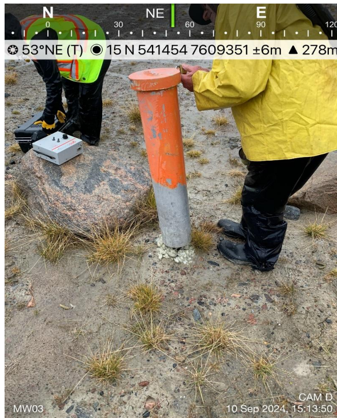
Photograph 2: Heaving at MW#3, exposed bentonite at base, casing on angle.
