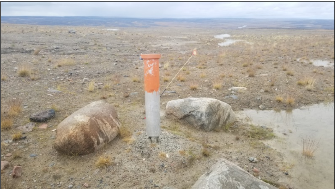
Photo 14: MW04 frost heaving.
