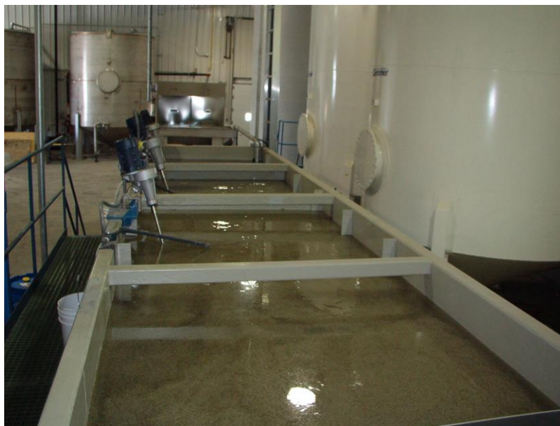
Project - Directline: TSS removal from waste water prior to secondary treatment. Included pre-screen, pH adjustment, polymer flocculation, clarification, sludge removal. Contact: Tony Ricciutto
