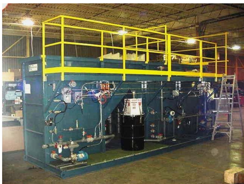
Project - Krispy Kernel: TSS removal from wash water prior to reuse or discharge. Included pre-screen, pH adjustment, polymer flocculation, clarification, sludge removal.
