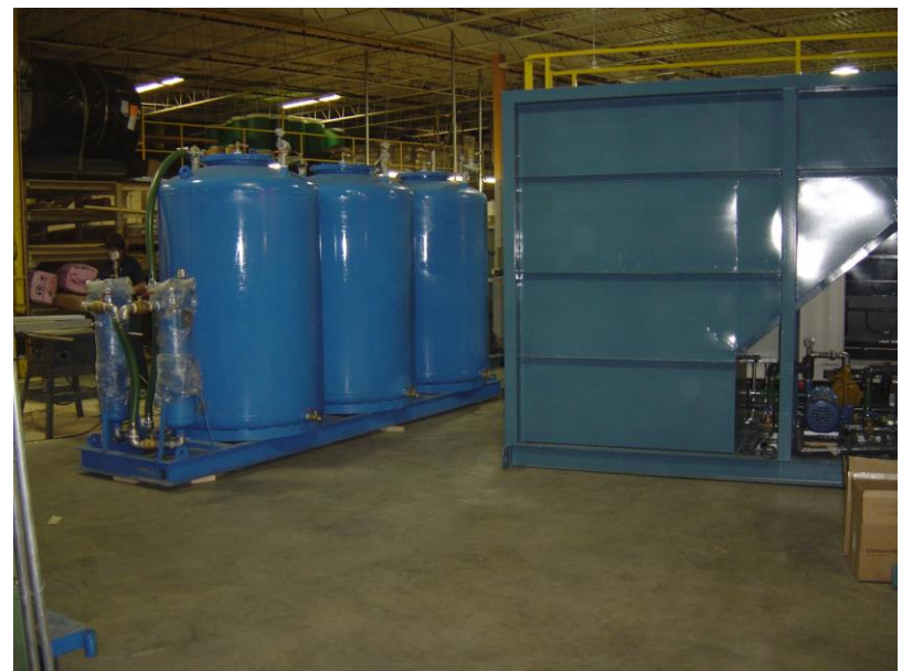
Project - Bennett: TSS removal from waste water prior to reuse or discharge. Included pre-screen, pH adjustment, polymer flocculation, clarification, sludge removal, media filtration.
