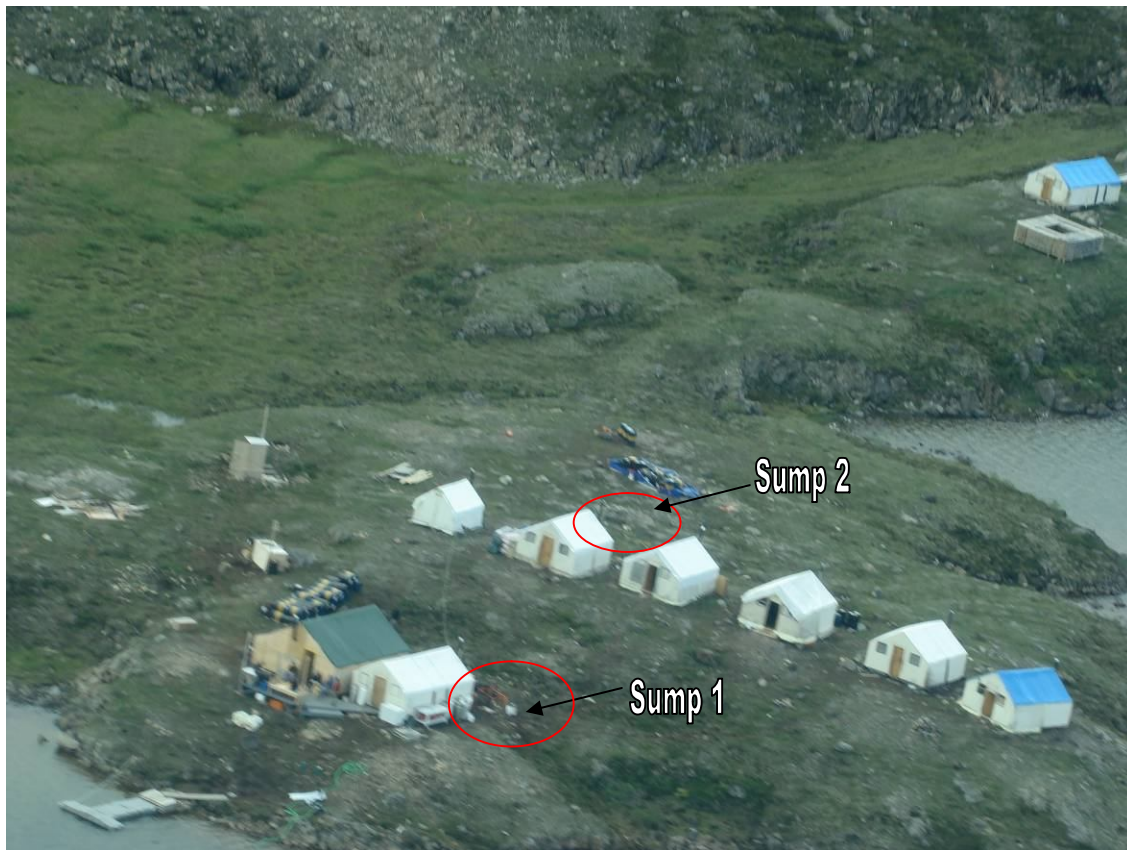
Photograph 2: Aerial view of Silvermet Camp. Sump 1 is near back corner of Dry tent; Sump 2 is located near main fuel cache. No secondary containment for helo refuelling area.
