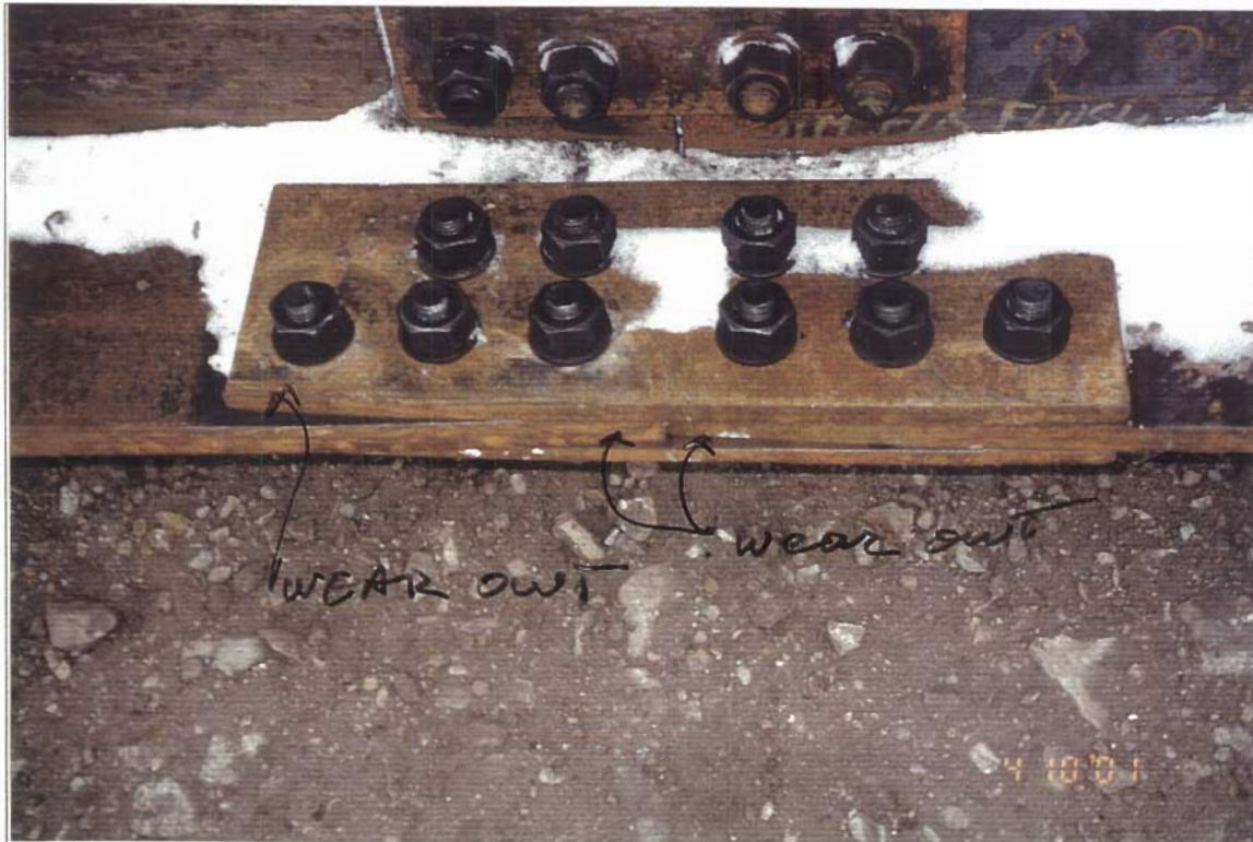
Bottom splice detail. Evidence of damage (wear out) on bottom flange due to dragging of girders on the ground during transportation.
