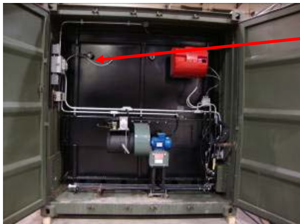
1. Primary Thermocouple (TC1)
