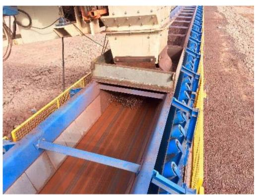
PHOTO 6 - Loading Ore onto the Conveyer belt
