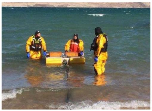
**PHOTO 4** Deploying a hydrocarbon skimming unit during the Marine Spill Response Training August 2015
