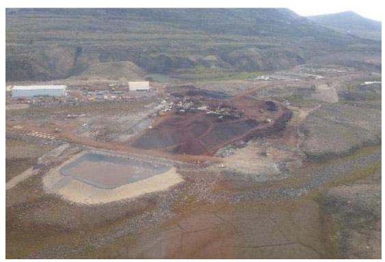
PHOTO 7 - Mary River Mine Site Crusher Pad Ore Stockpile and Sedimentation Pond
