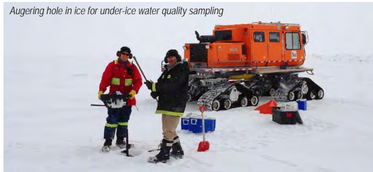
Augering hole in ice for under-ice water quality sampling
