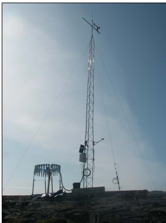
Plate 2.1-2. Doris meteorology station after being upgraded to a 10 m tower.
