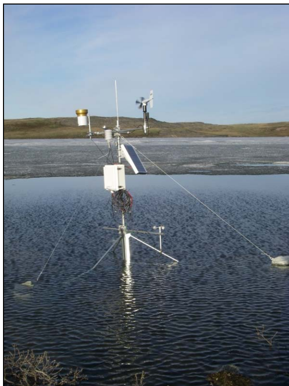
Plate 2.1-4. The Doris Lake micro-meteorology (evaporation) station in July 2009.
