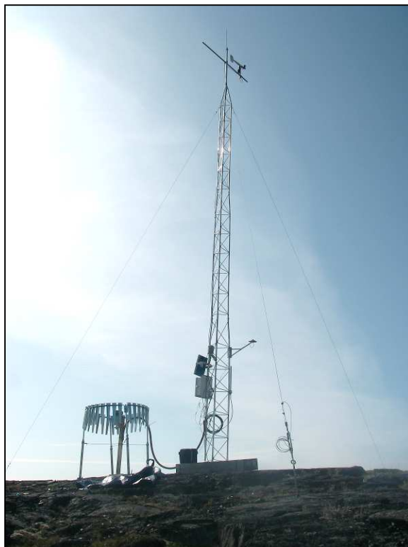
Plate 2.1-1. Doris meteorological station after being upgraded to a 10 m tower on August 13, 2009.
