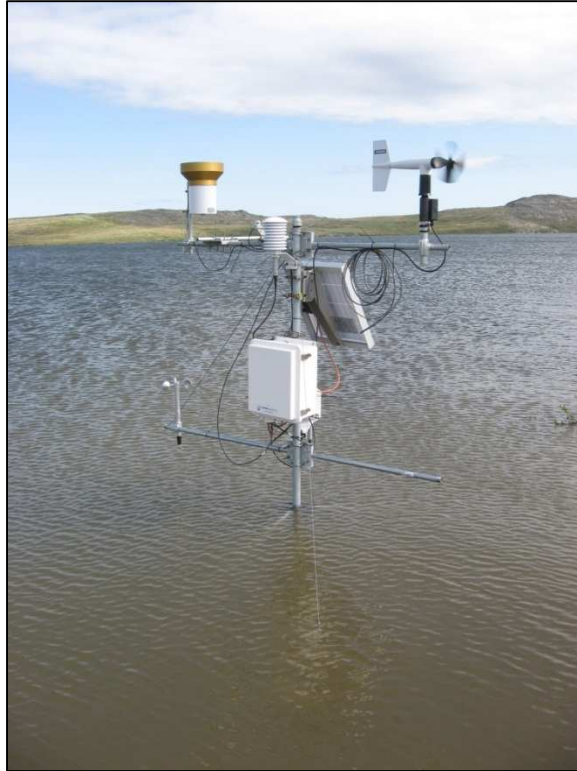
Plate 2.2-1. The Doris Lake micro-meteorological (evaporation) station in July 2012.
