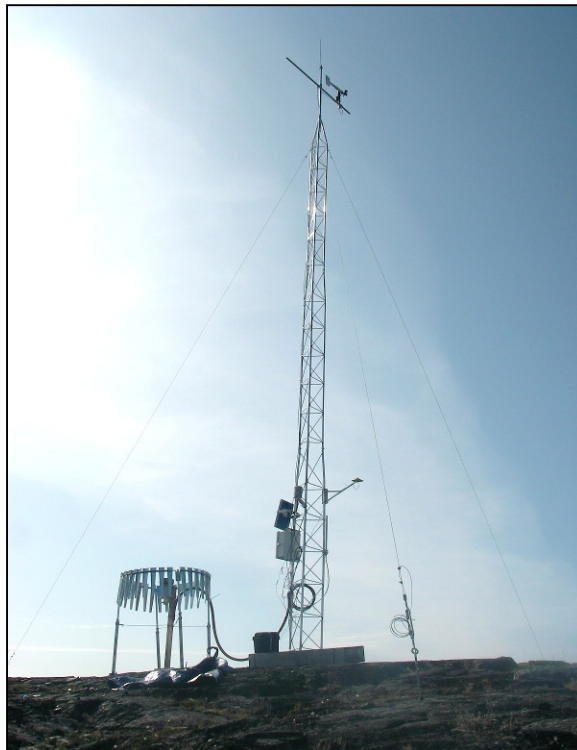
Plate 2.1-1. Doris meteorological station after being upgraded to a 10 m tower on August 13, 2009.
