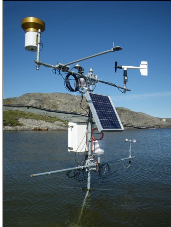
Plate 2.2-1. The Doris Lake micro-meteorological (evaporation) station in July 2013.
