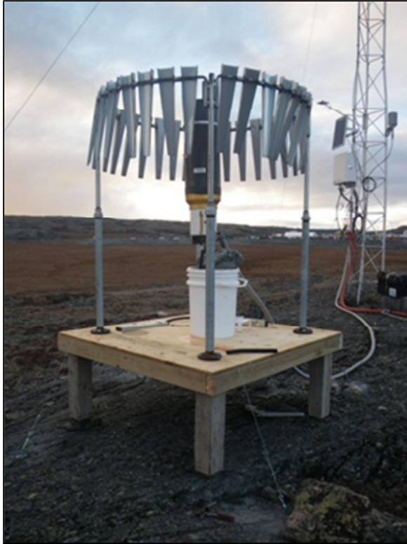
Plate 2.1-2. The newly installed platform for the alter wind screen and tipping bucket rain gauge. The TBRG has the winter precipitation adapter installed on it, September 29, 2013.
