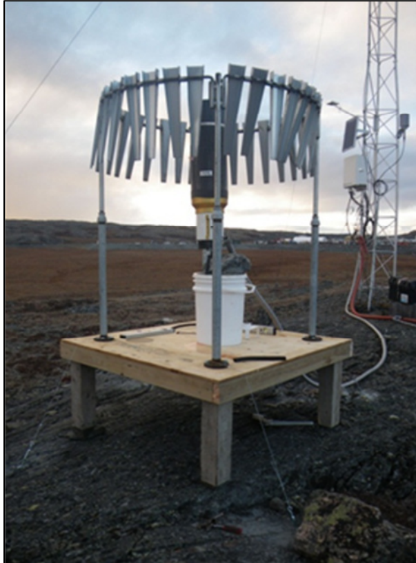
Plate 2.1-2. The newly installed platform for the alter wind screen and tipping bucket rain gauge, September 29, 2013. The TBRG includes a winter precipitation adapter.
