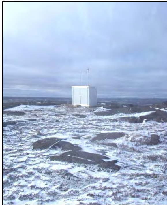
Plate 2.1-2. Temperature controlled shelter housing the Partisol ambient air samplers, late August 2009.
