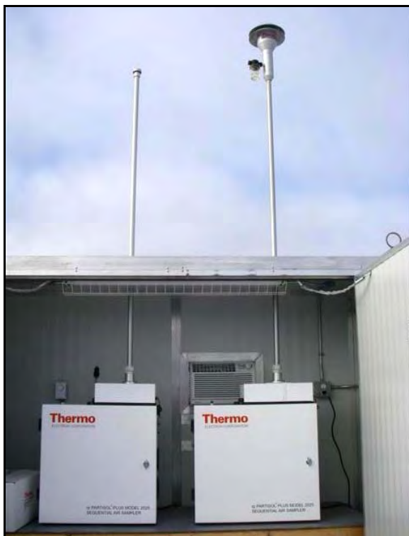
Plate 2.1-3. Inside the temperature controlled shelter the Partisol sampler for TSP is shown on the left and the PM10/PM2.5 sampler is on right.
