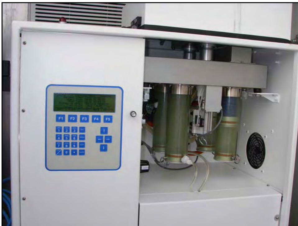
Plate 2.1-4. The new Partisol air sampler filters are contained in a magazine on the left side of the unit. The filters laden with suspended particulate matter are contained in a magazine on the right side of the unit.
