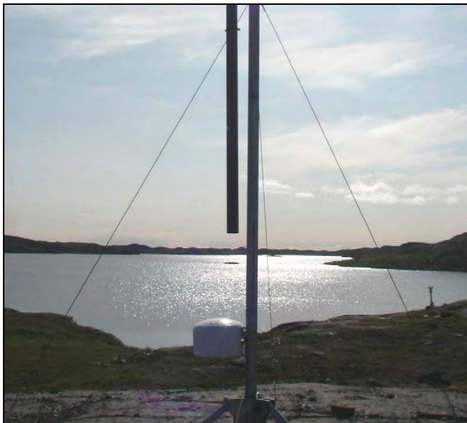
Plate 3.1-1. The white circular device shown in this photo is the passive air sampling system near the Doris automated meteorological station.
