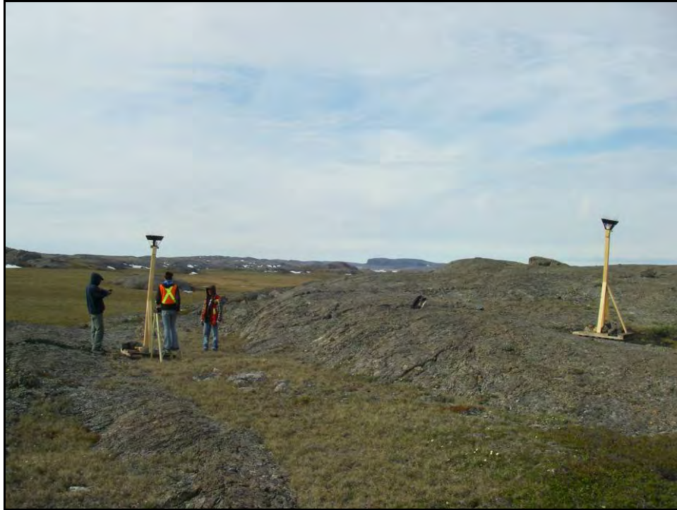
Plate 2.2-1. Dustfall monitoring station three near the Doris project site. For locations using the ASTM (2004) method two sample containers are required to provide a sufficient volume of sample for the various parameters (e.g. particulate, anions, cations, total metals). Locations using the Alberta Environment (AMD 1989) method only require one collector.
