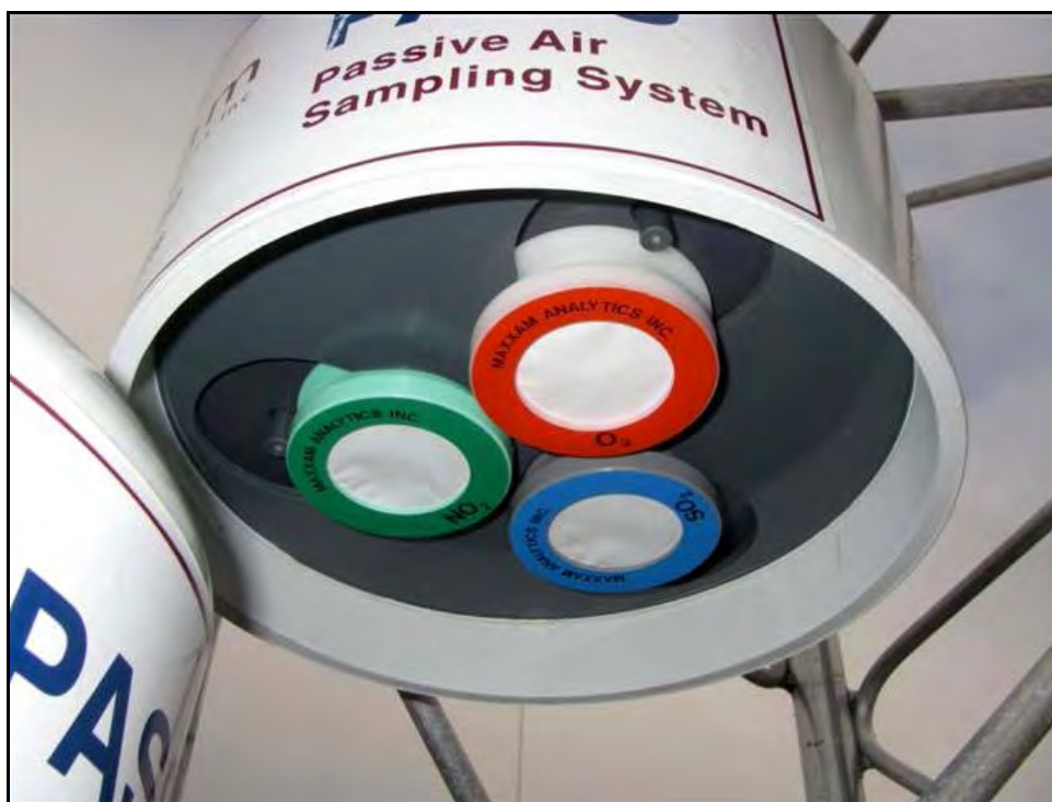
Plate 3.2-1. Passive air samplers under a rain shelter.
