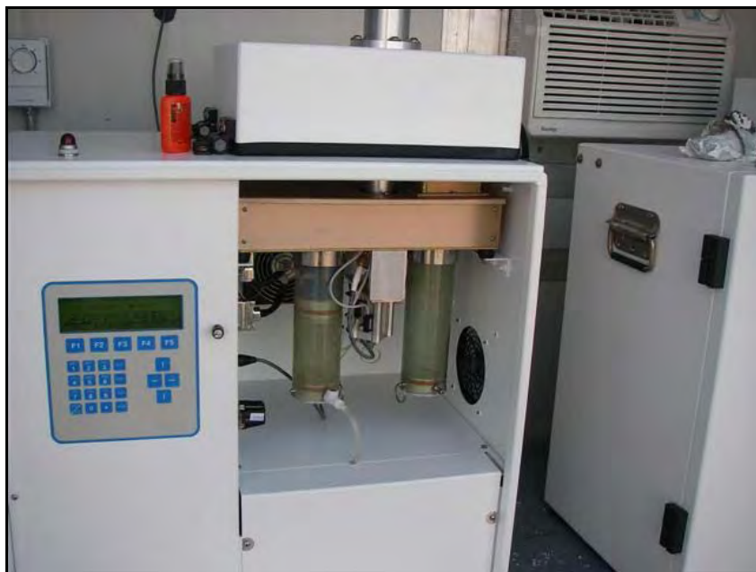
Plate 2.3-1. Thermo 2025 TSP Sampler. The left hand magazine contains new filters and the right hand magazine contains used filters.
