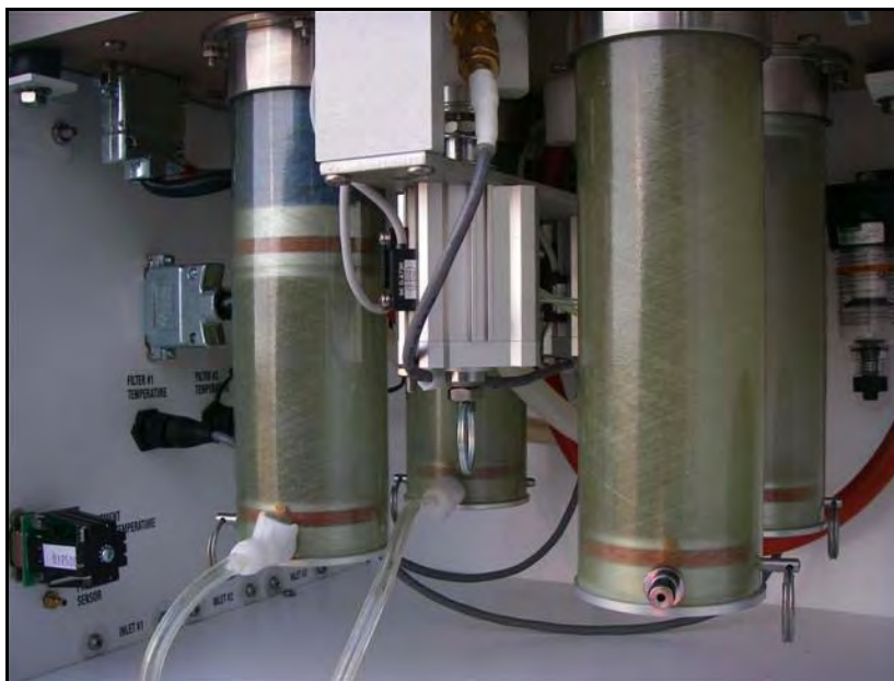
Plate 2.2-1A. 2025D Sequential Dichotomous ambient air quality sampler - Left side magazine loaded with new filters and right side magazine for used filters. The front magazines are for PM10 and the back magazines are for PM2.5.
