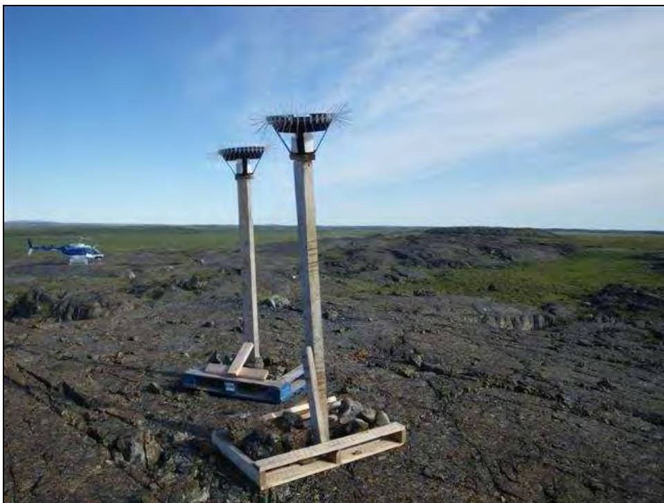
Plate 2.2-1. Dustfall monitoring station (DF4) near the Doris project site. For locations using the ASTM (2004) method two sample containers are required to provide a sufficient volume of sample for the various parameters (e.g. particulate, anions, cations, total metals). Locations using the Alberta Environment (AMD 1989) method only require one collector.
