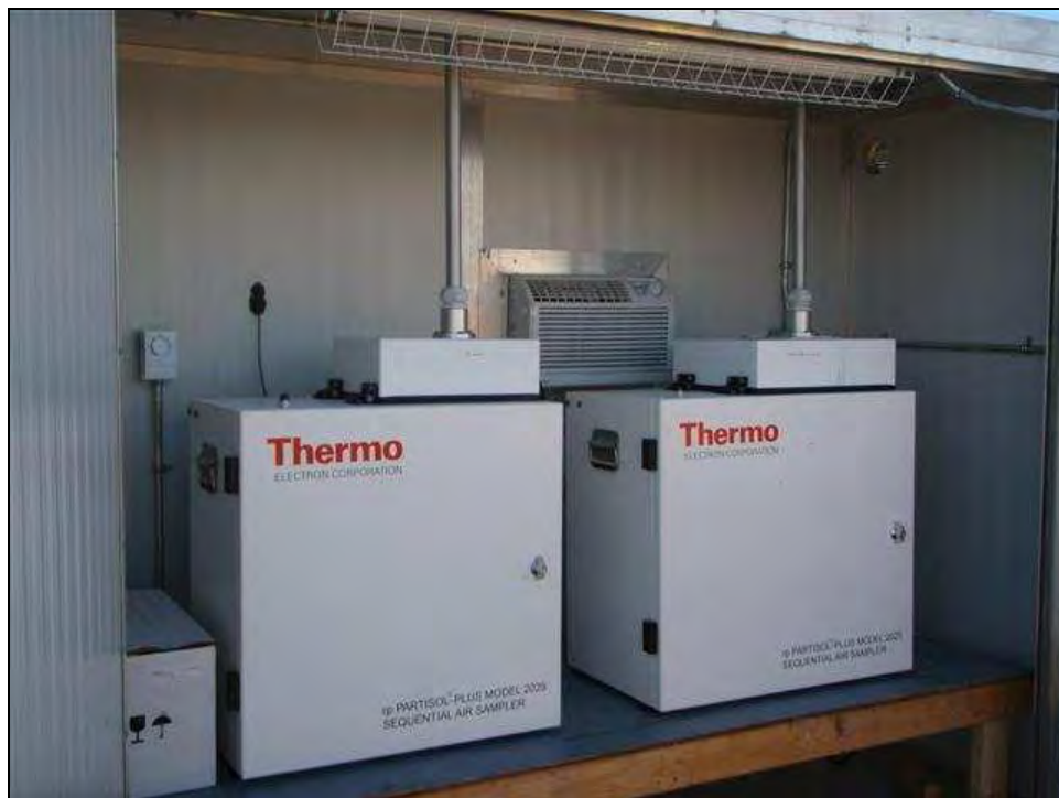
Plate 2.1-3. Inside the temperature controlled shelter the Partisol sampler for TSP is shown on the left and the PM 10 /PM 2.5 sampler is on right.
