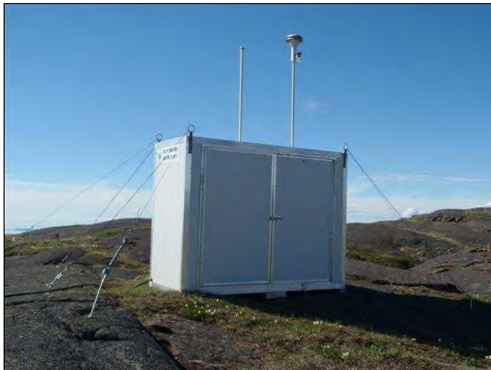
Plate 2.1-2. Temperature controlled shelter housing the Partisol ambient air samplers, early July 2010.
