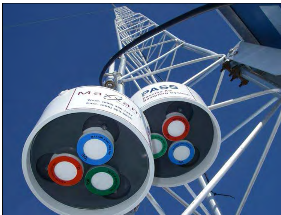
Plate 3.1-1. The white circular device shown in this photo is the passive air sampling system on the Boston automated meteorological station.
