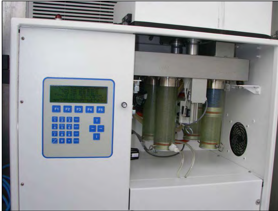
Plate 2.1-4. The Partisol air sampler filters are contained in a magazine on the left side of the unit. The filters laden with suspended particulate matter are contained in a magazine on the right side of the unit ( PM_{10} at front and PM_{2.5} at rear).
