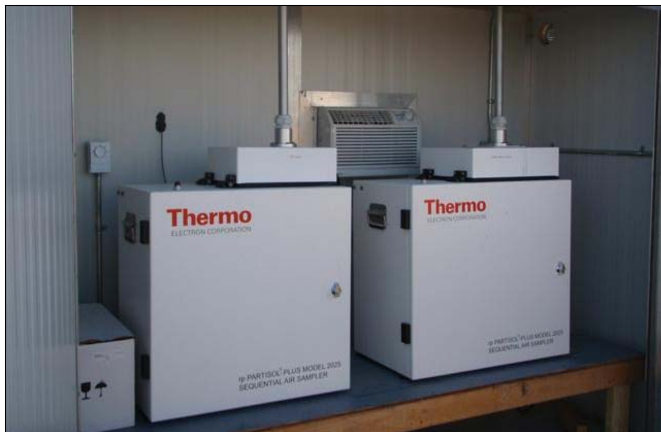
Plate 2.1-3. Inside the temperature controlled shelter the Partisol sampler for TSP is shown on the left and the PM 10 /PM 2.5 sampler is on right.
