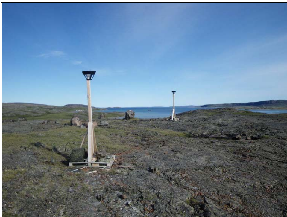
Plate 2.2-1. Example of a dustfall monitoring station (DF1) near the Doris North Project site which uses the ASTM monitoring method.
