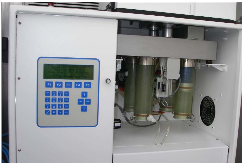
Plate 2.1-4. The Partisol air sampler filters are contained in a magazine on the left side of the unit. The filters laden with suspended particulate matter are contained in a magazine on the right side of the unit ( PM_{10} at front and PM_{2.5} at rear).
