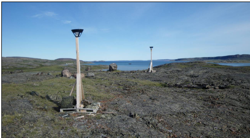
Plate 2.2-1. Example of a dustfall monitoring station (DF1) located approximately 1 km west of the Roberts Bay laydown area which uses the ASTM monitoring method.
