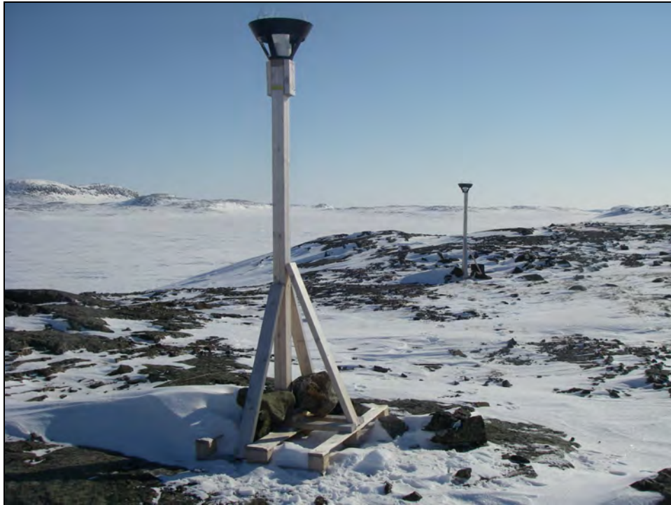
Plate 2.2-1. Example of a dustfall monitoring station near the Doris North Project site which uses the ASTM monitoring method.
