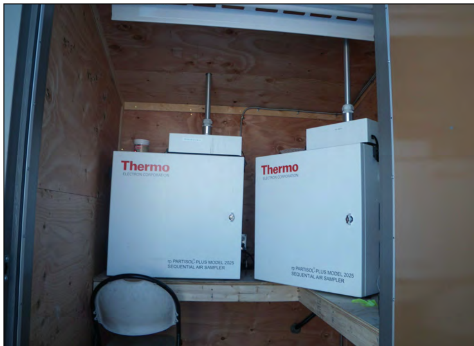
Plate 2.1-3. Inside the temperature controlled shelter. The Partisol sampler for TSP is shown on the right and the PM_{10}/PM_{2.5} sampler is on the left.
