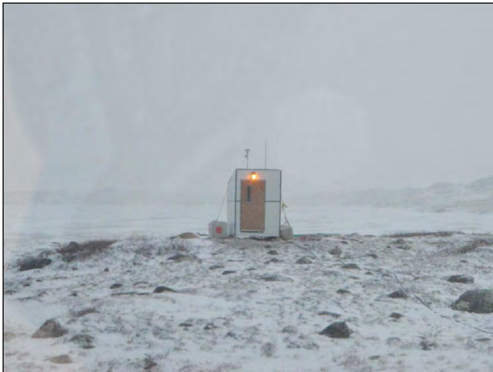
Plate 2.1-2. Temperature controlled shelter housing the Partisol ambient air samplers, October 2011.
