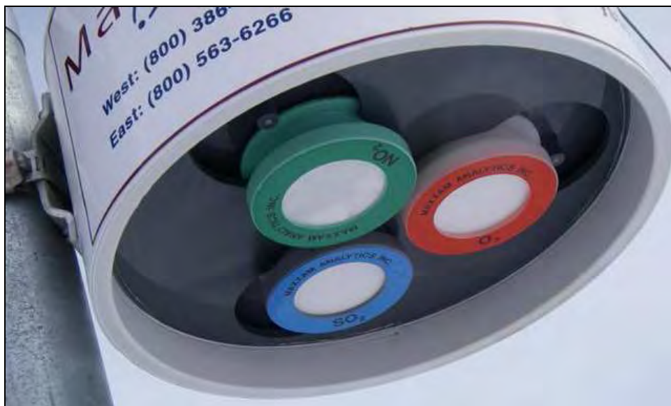
Plate 3.2-1. Passive air samplers under a rain shelter at Doris meteorological station.
