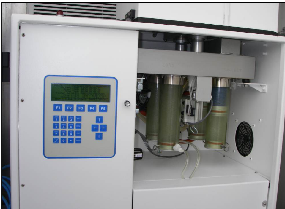
Plate 2.2-2. The Partisol air sampler filters are contained in a magazine on the left side of the unit. The filters laden with suspended particulate matter are contained in a magazine on the right side of the unit (PM 10 at front and PM 2.5 at rear).
