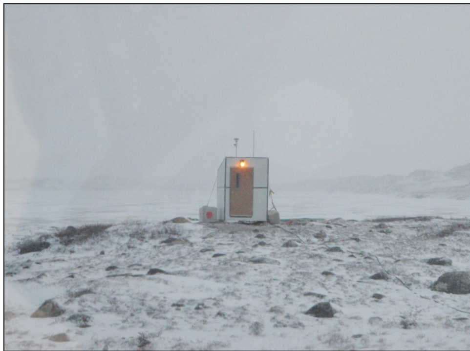
Plate 2.1-2. Temperature-controlled shelter housing the Partisol samplers, October 2011.
