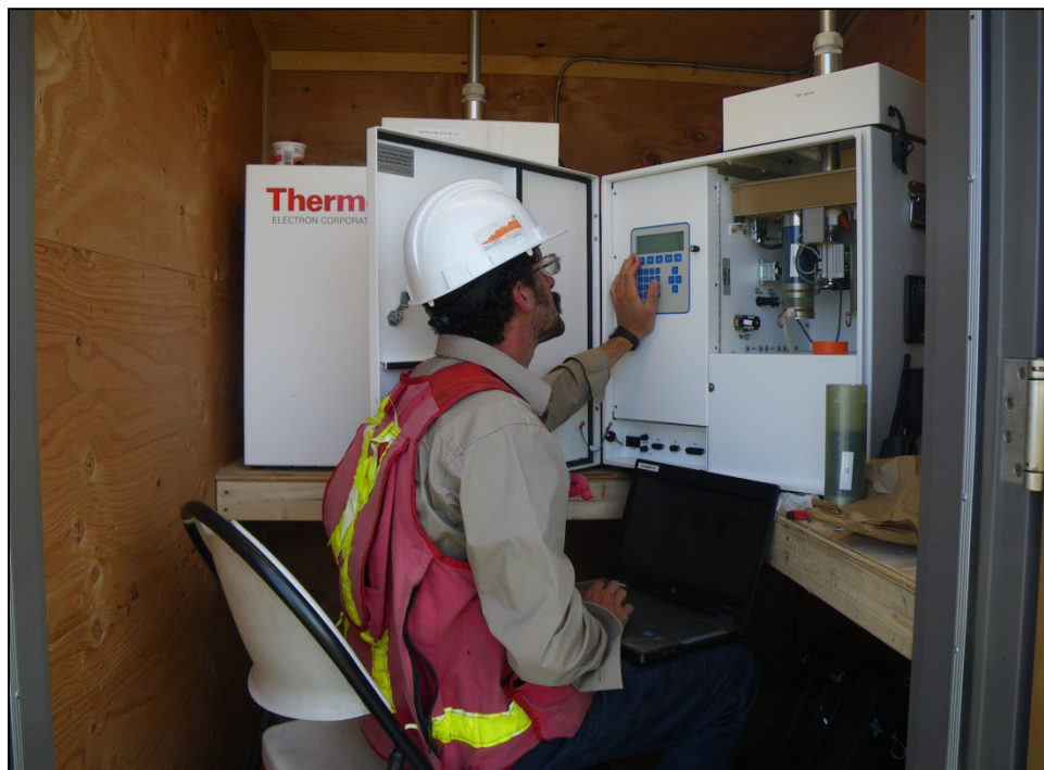
Plate 2.2-1. Inside the temperature controlled shelter. The Partisol sampler for TSP is shown on the right and the PM 10 /PM 2.5 sampler is on the left, July 2013.
