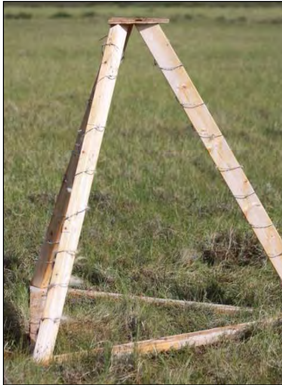
Plate 2.1-1. Tripod design used during 2010 grizzly bear DNA study.
