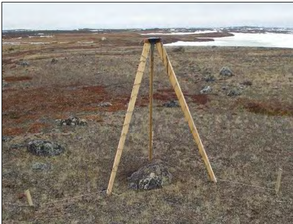
Plate 2.2-2. Fold-up hair snagging tripod anchored with wooden stakes.
