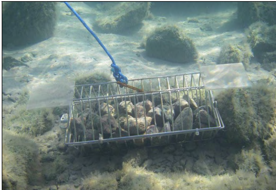
Plate 2.2-3. Artificial substrate sampler with attached periphyton Plexiglas plates submerged on a shoal in the Reference Bay, Doris North Project (2009).
