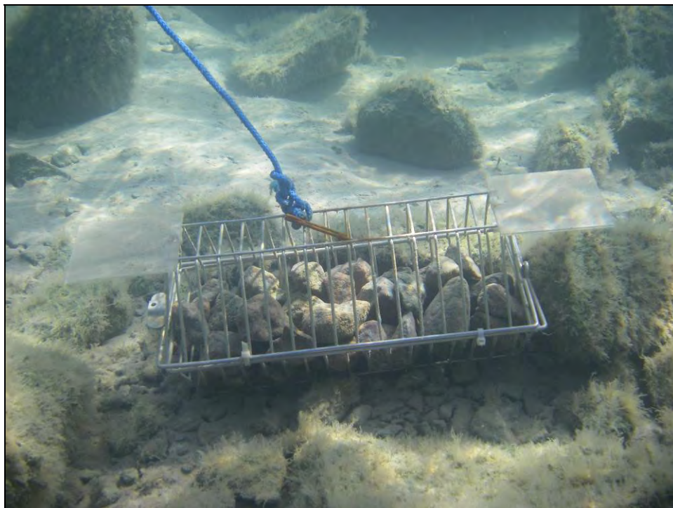
Plate 2.2-3. Artificial substrate sampler with attached periphyton Plexiglas plates submerged on a shoal in the Reference Bay, Hope Bay Belt Project, 2009.
